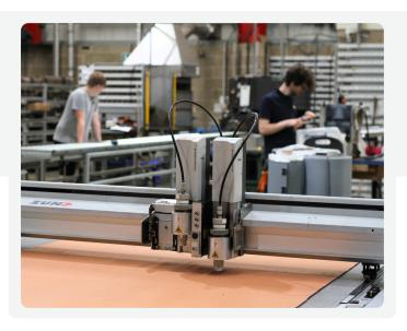
Our CNC cutting machine can accommodate sheets up to 2m wide and, when linked to a conveyor, can cut to any length required (subject to the length of the raw material available).
